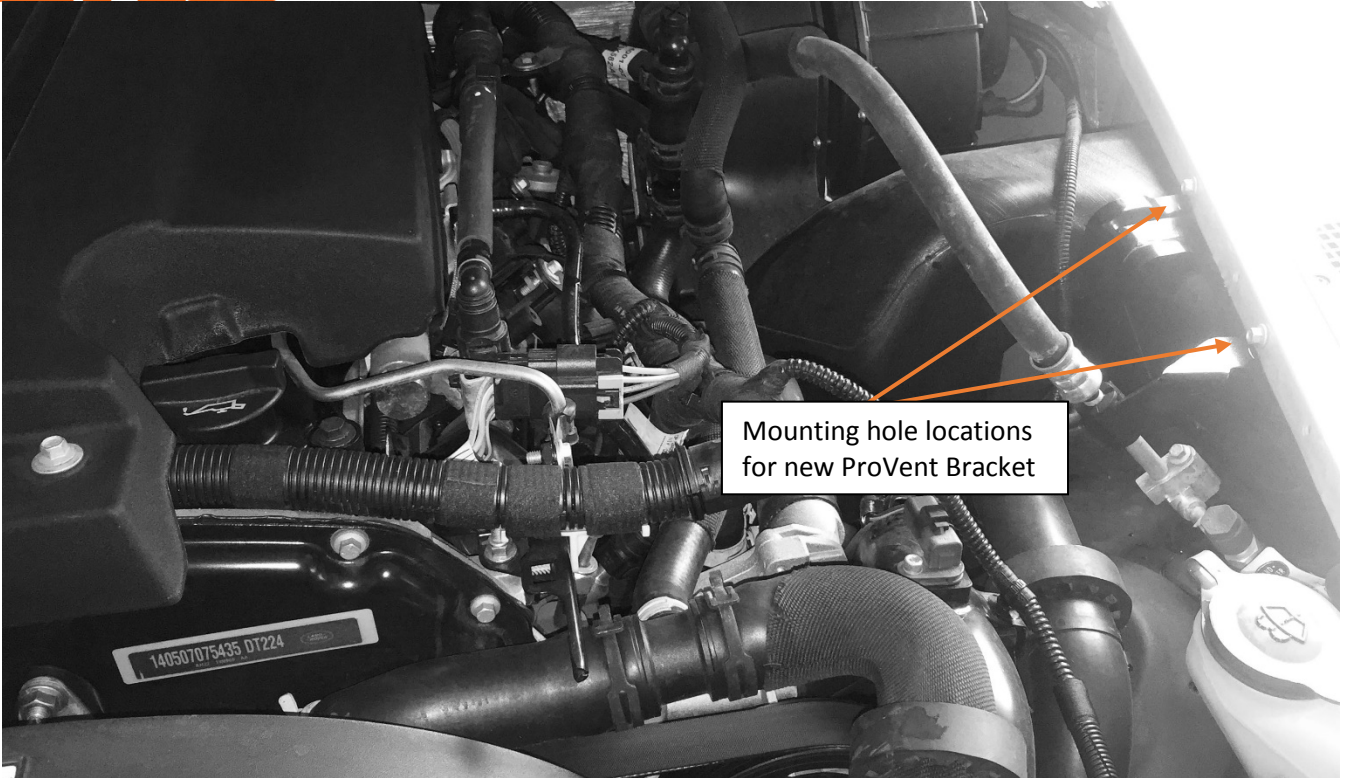
Top down view: image shows new ProVent bracket location, the installation reuses existing bolts
