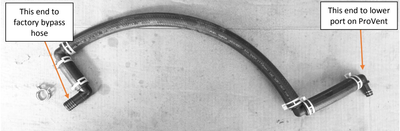
Assembled Return Hose. From left to right the hose lengths are 55mm, 600mm and 125mm
