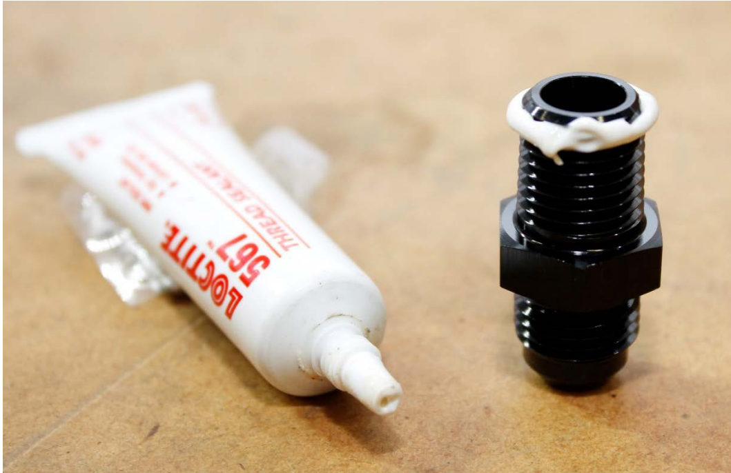
Fitting with Loctite applied
