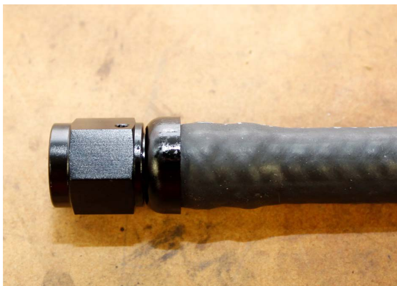
Correctly installed push lock fitting
