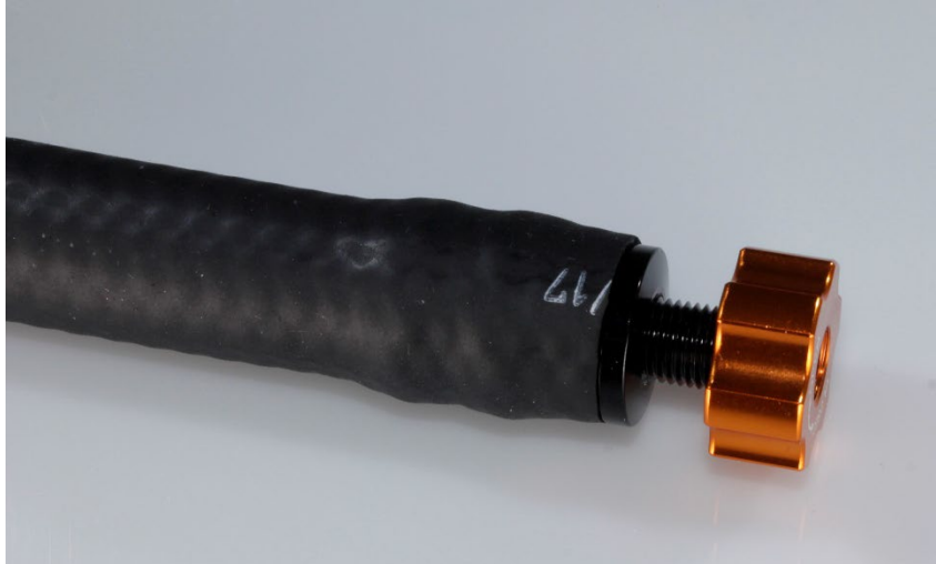
Hose tail and tap assembly inserted into 12mm hose, secured with a clamp
