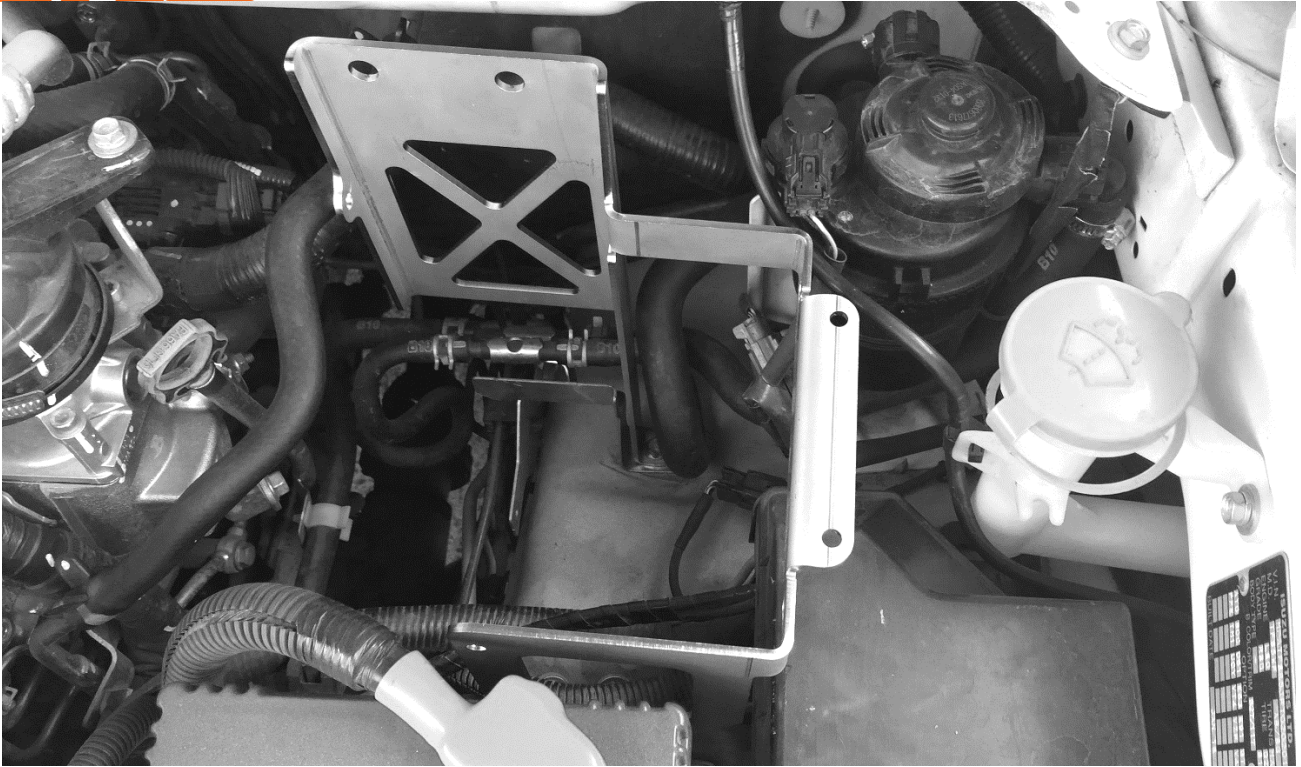
D-Max Engine Bay- Rear Passenger Side with new bracket installed
