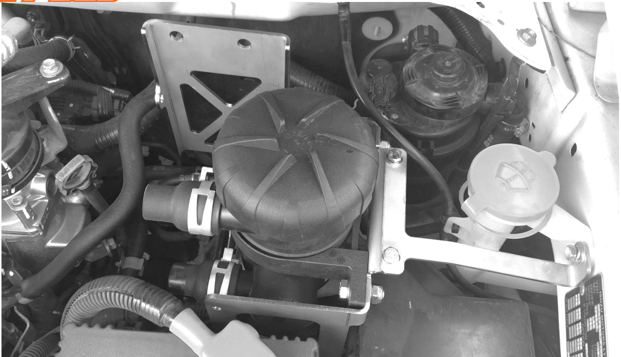
ProVent 200 bolted in place at correct orientation with first support bracket in place. 25-16mm reducing couplers and clamps are also installed in this picture
