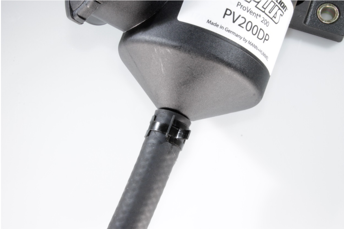
ProVent® 200 with 12mm hose connected and secured with 12-20mm clamp
