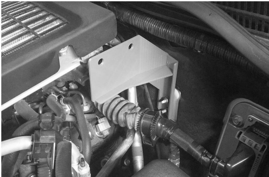
New bracket secured in place, note prototype bracket in place, not production version
