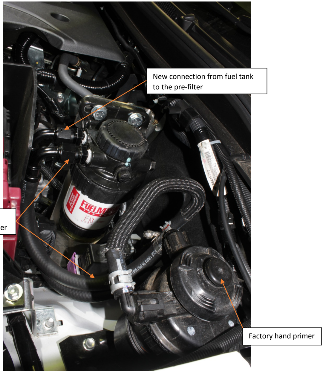
image showing prefilter connection and hose routing
