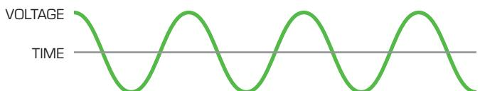
REDARC Pure Sine Wave Inverters are the safest choice for using common household appliances on the road as they give you an output almost identical to household mains power.
