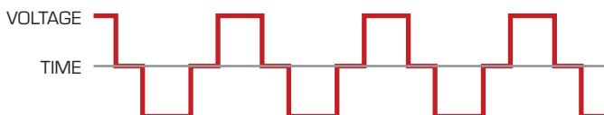
Cheaper inverters try to imitate a sine wave by 'chopping off' the corners of a sine wave. Modified sine wave inverters can often lead to appliances overheating due to faster switching times on each polarity change, which stresses appliances and devices.
