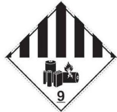
Use Class 9 Miscellaneous Dangerous Goods and UN Identification labels for transportation of Lithium-ion batteries which are assigned Class 9. Refer to relevant transportation documents. Lithium and Lithium-ion cells and batteries are regulated in the U.S. in accordance with Part 49 of the Code of Federal Regulations, (49 CFR Sections 105-180) of the U.S. Hazardous Materials Regulations.
