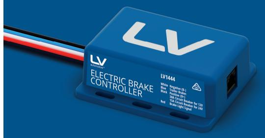
The LV1444 electric trailer brake controller provides smooth application of a connected electric braking system. Brake actuation is automatic, user-definable and overridable via a discrete, multi-positionable control. Designed to suit both 12 and 24V tow vehicle electrical systems, the LV1444 can operate 1-3 axle 12V electric brake systems.
