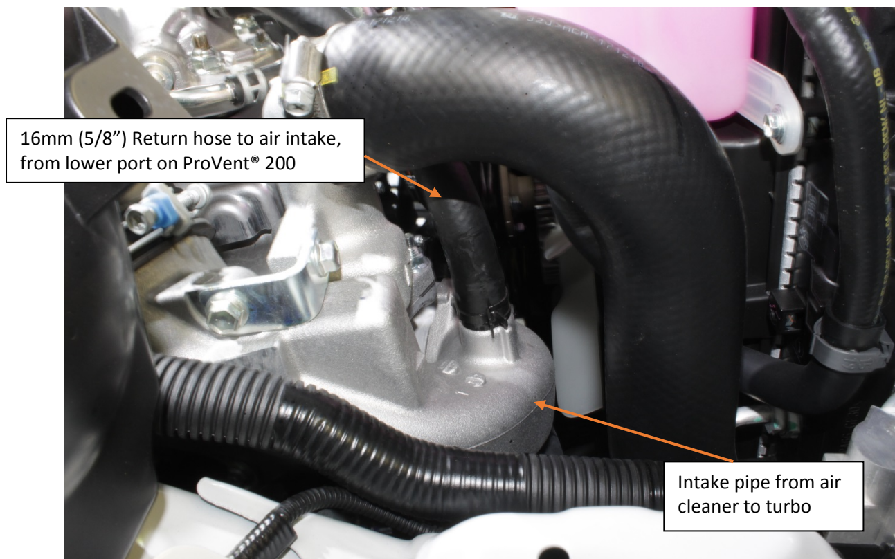
Hose configuration in Land Cruiser Prado 155 Series 1GD-FTV with ProVent® 200 installed
