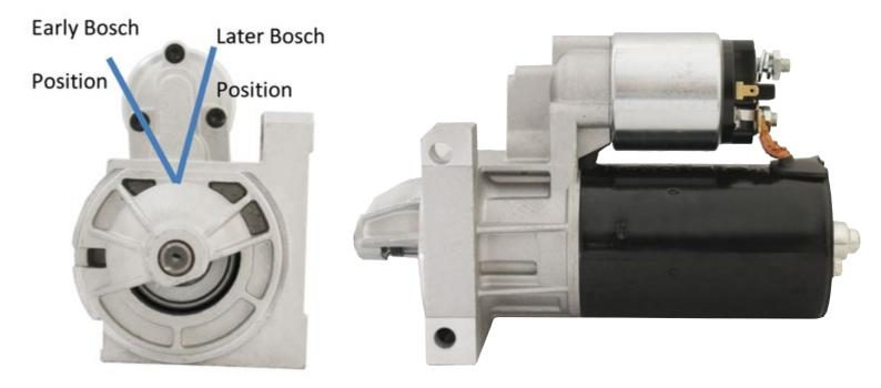
SNB010 is a Holden V8 aftermarket starter to suit "Red, Blue and Black" Holden non Injected 4.2 and 5.0 litre motors which replaces 2 original Bosch starters that were slightly different.
