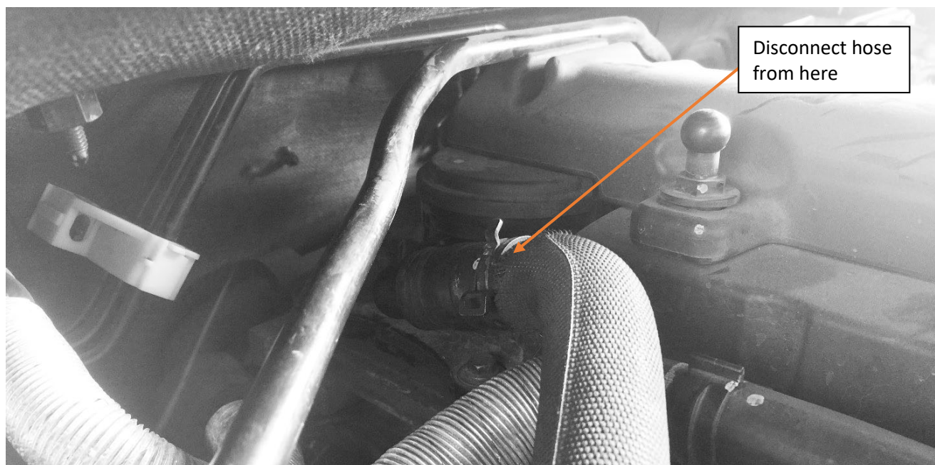
Factory bypass hose location
