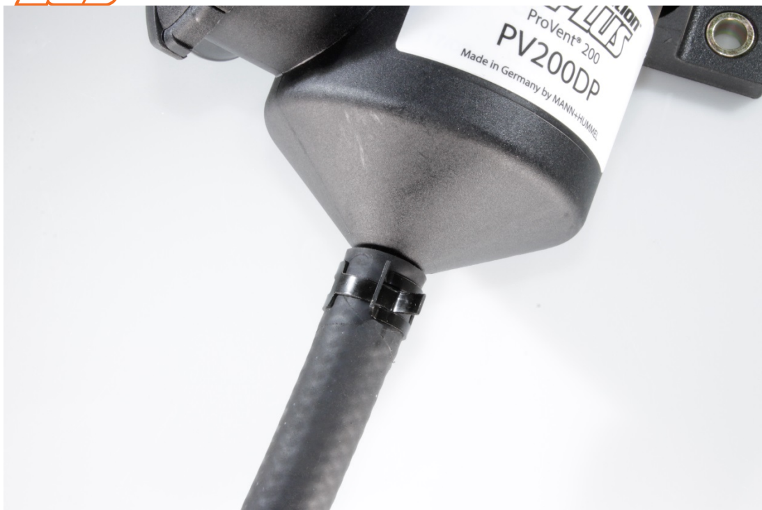
Provent 200 with 12mm hose connected and secured with 18-20mm clamp
