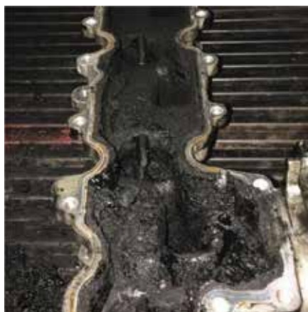
Mitsubishi Triton Blocked Inlet Manifold
