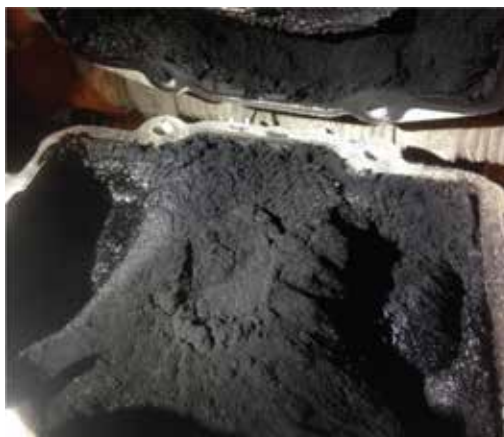
Toyota 1VD-FTV Blocked Inlet Manifold
