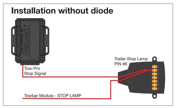
For older vehicles, not supplied with driver aids e.g. Cruise, Traction or Stability Control, Brake/Throttle Override
