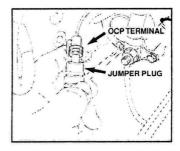
Tie off the OCP terminal and plug to the main wire harness to prevent separation due to vibration.
