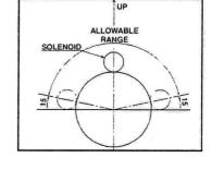
NOTE: The solenoid should be mounted upward over 15 degrees of horizontal. Water, oil dust and other foreign material may enter the starter if the solenoid is not mounted properly. Starter operation failure will result over a period of time.
