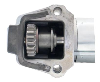
SNA008 and SNA013 are Pad Mount starter motors fitted to Ford Transit 2.4 Litre Turbo Diesel Motors that utilize a Dual Mass Flywheel. The Dual mass flywheel, as it wears tends to "throw out" metal particles and dust that has an adverse effect on the way this starter operates by contaminating the two drive end shafts that are co-mounted parallel in the end housing.
