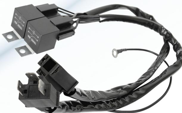
Most aftermarket LED Headlights require a positive switched feed to activate the light. Because there are a few vehicles out there that switch earth instead of a positive this will cause the LED headlight to not activate. These Headlight Adaptor Harness Kits solve that problem by changing the earth to a positive supply.
