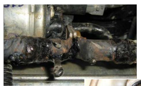
This damage to the Solenoid Stud is **NOT** a manufacturing defect but caused by external heat and any starter returned with this problem will **NOT** be covered by warranty regardless of time fitted.
