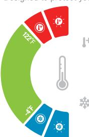
**Hot LED indicator.** Designed to indicate when internal battery approaches high temperatures.
